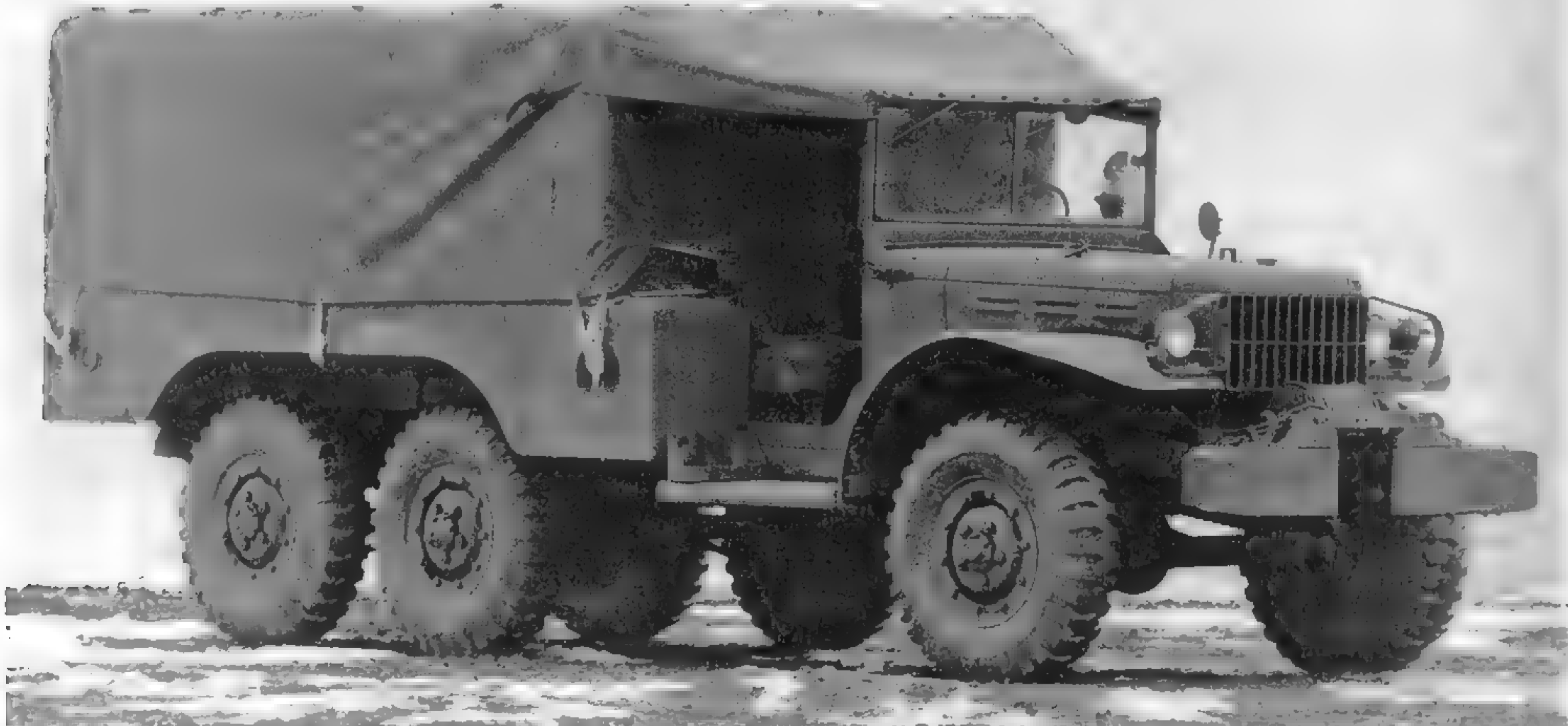
The WC-63 was essentially the same truck as the WC-62, differing only in its PTO-driven Braden MU-2 winch. Initially, the winch capacity was rated at 5,000-lbs., but an increase in wire rope size from 3/8 to 7/16 in. allowed the rating to be raised to 7,500 lbs. (U.S. Army photo)
